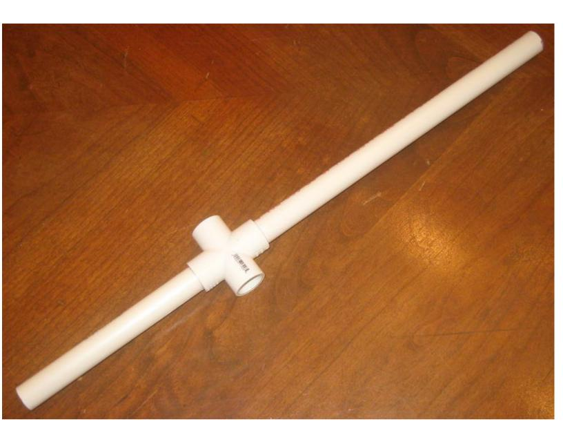
Glue the two remaining cross connectors on to each end of the assembly from step 3. Make sure to align the cross connectors. An easy way to align the connectors is to place them on a flat surface before the glue sets and twist them to be flat with the surface.
