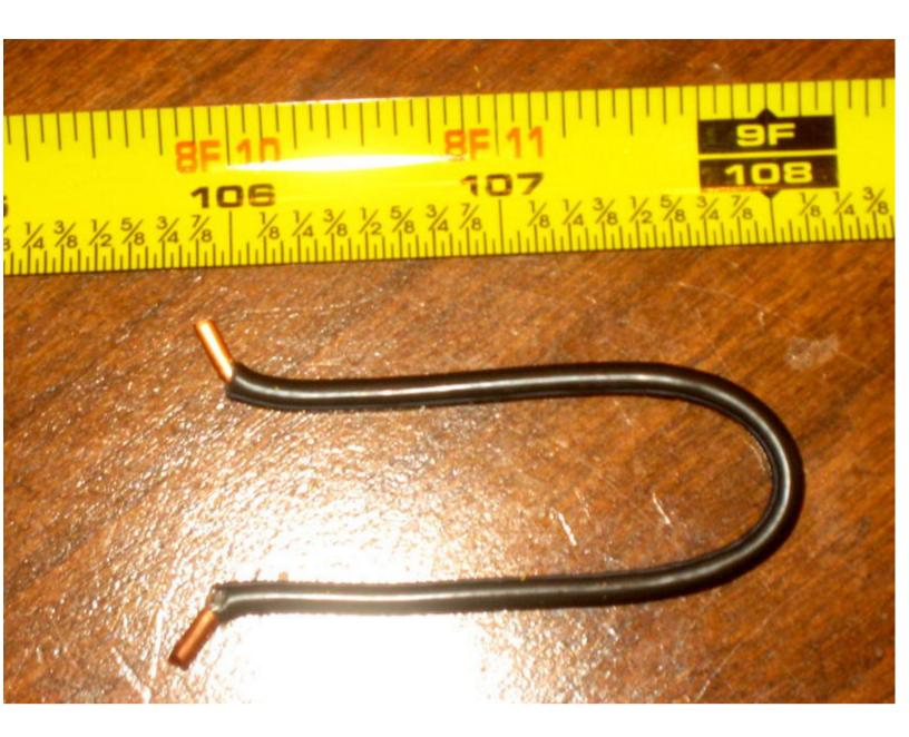
Scrape about 1/4 inch of paint off of the two remaining pieces of tape rule from the untaped ends. Tin the bare areas, then attach the hairpin match and coax wire.
