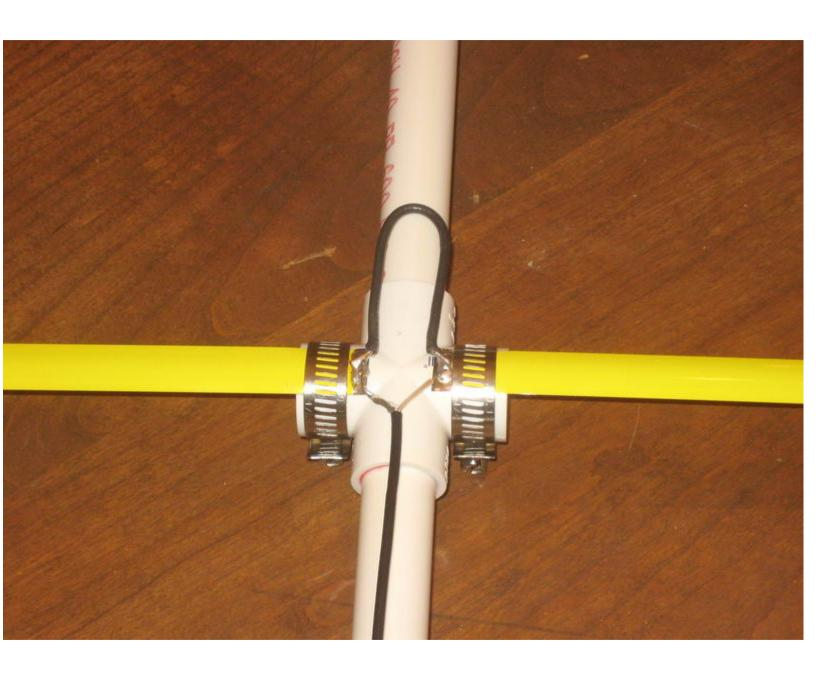
Secure the coax wire to the boom with a zip tie or black tape. The antenna is now ready to use.
