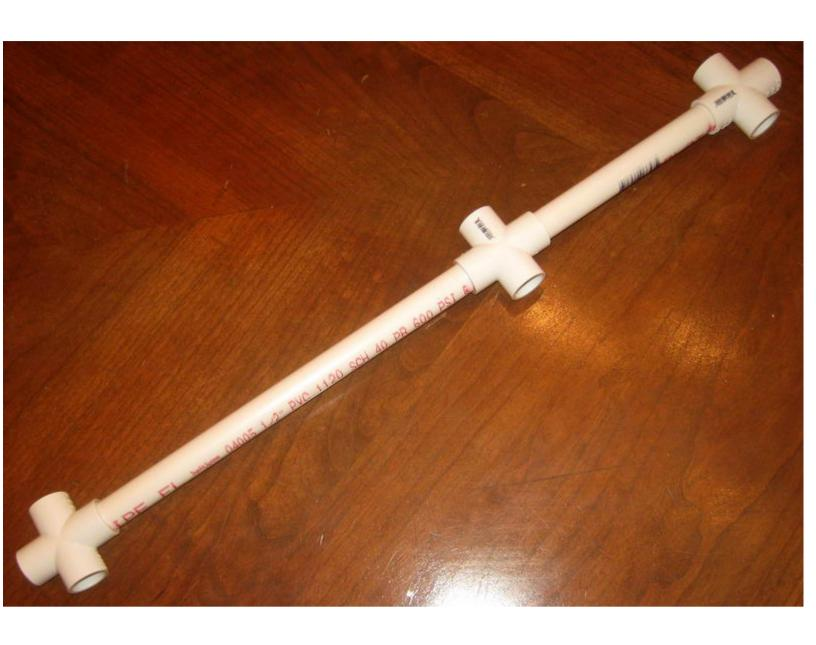
Glue the two short pieces with end caps to each end of the assembly from step 4.
