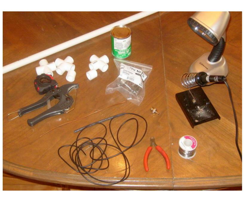
Cut an  $11\ 1/2$  inch, a 7 inch, and two 5 inch pieces of PVC pipe. Before cutting the pipe, it might be helpful to measure and mark the length using a sharpie black marker.
