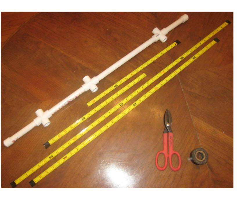
Attach the longest (41 3/8 inchh) piece of tape rule to the cross connector closest to the center cross connector. It will be helpful to mark the center point (20 11/16 inches) with a black sharpie marker. Position the tape over the cross connector, so the curve of the tape rule is similar to the curve on the cross connector. Center and secure the element with hose clamps on each side as pictured.
